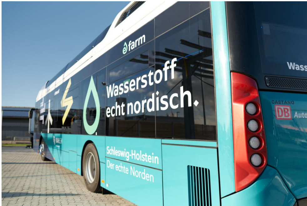
Caption 1: The latest technology and a range of 400 km enable flexible use of the fuel cell buses in Autokraft's route network.
