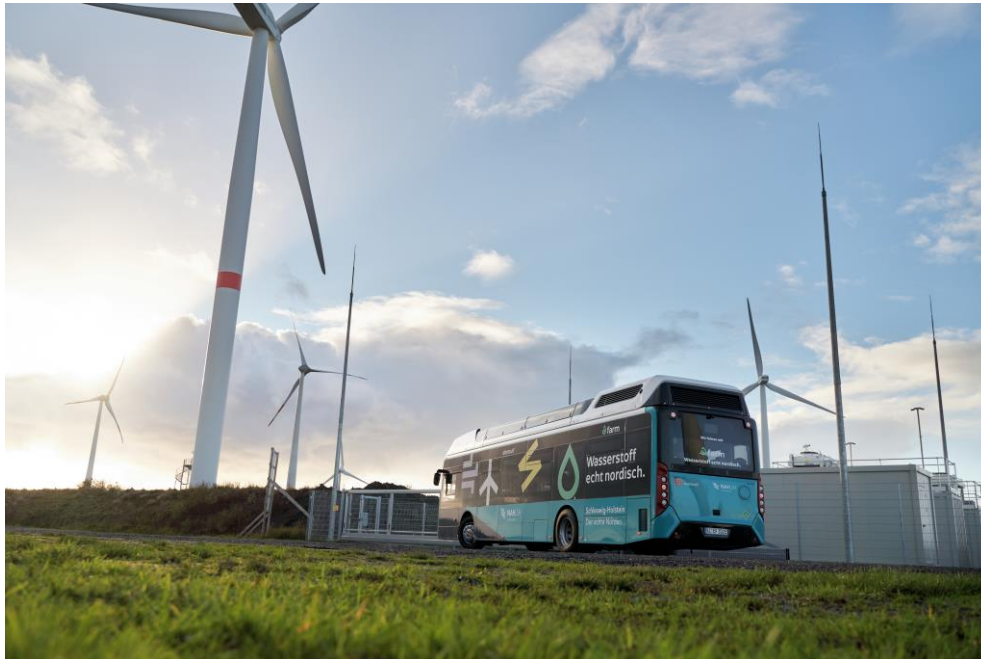
Capion 2: One of the fuel cell buses in front of the production plant in Bosbüll. Here, the hydrogen for the drive is produced from wind power.
